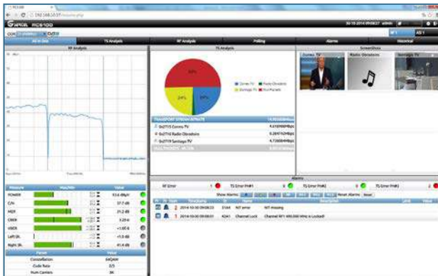
All in One Shows an overview of the channel status on one screen. It shows spectrum, services, measures, alarms, Pids. All integrated in a single view for quick analysis.
