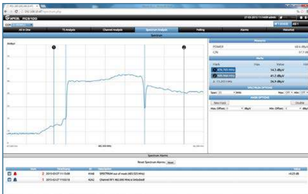
Full Spectrum (opt.) Represents realtime spectrum of the monitored channel with detailed measures Mask, max. hold and min. hold features.
