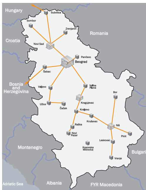
Figure 83. Leased Intercity Optical Links – Current State
