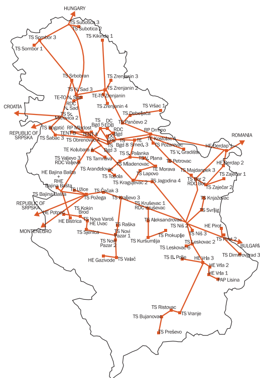
Figure 76. “Electric Power Industry of Serbia” Optical Network
