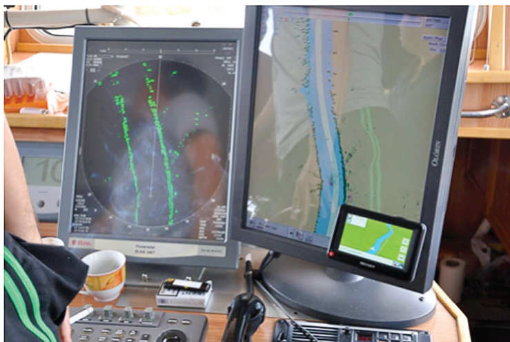
Figure 92: ECDIS display on the command bridge and the position of the vessel on the electronic navigation map
